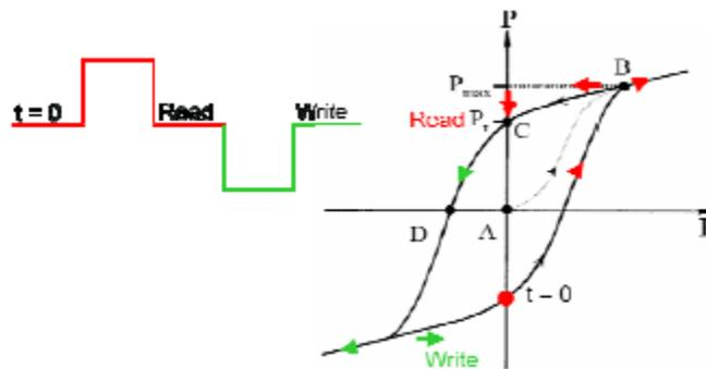
Figure 6: FRAM Write/Read cycle
