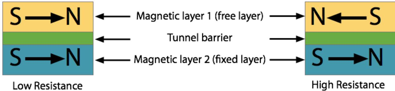
Figure 2: MRAM Magnetic Tunnel Junction (MTJ) Storage Element
