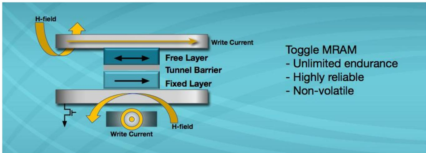
Figure 1: Magnetic Tunnel Junction (MTJ)
